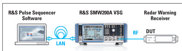
▲ Fig. 1 The R&S SMW200A VSG with R&S Pulse Sequencer PC software provides a compact, powerful radar simulator for the lab.
