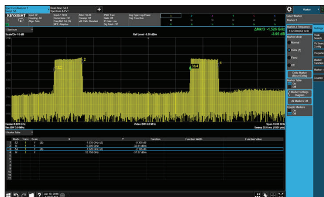
▲ Fig. 2 Signal generator output with two chirped radar emitters, 1.5 GHz wide and 7 GHz apart.
