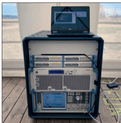
▲ Fig. 3 At an OTA demonstration at Tartu Airport in Estonia, the signal generators and amplifier were mounted in a small rack, with the R&S Pulse Sequencer software running on a commercial laptop.
